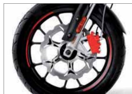
Frenos radiales, horquilla invertida de 41 mm y discos Wave/Freni radiali e forcella rovesciata. Ø 41 mm e dischi Wave/Radial brakes and upside down fork. Ø41mm and Wave disks.
